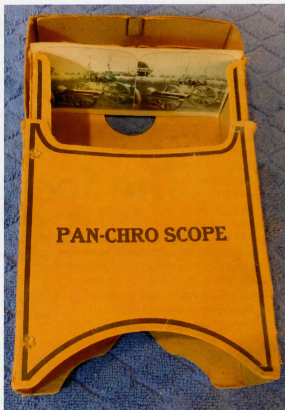
Top view of the shoe box like Pan-Chro Scope cardboard viewer, with stereo card inserted for viewing. The lens holder fits into the body at the front and the slide holder is placed into the body at the rear and is moved backward or forward for focus. This is the only known Pan-Chro Scope viewer in existence. (Photo courtesy of Doug Jordan)
