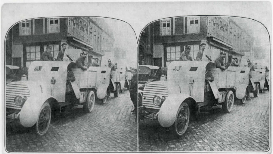
Pan Chro Scope Corp. 1918 Series 2, No. 27, "Armored Cars of the French Army in active service." A 1909 model Automitrailuses Hotchkis armored car with an unusual front plate protecting the driver. Usually with this model, the driver just had a small armored plate over his head protecting him and no front armor.
