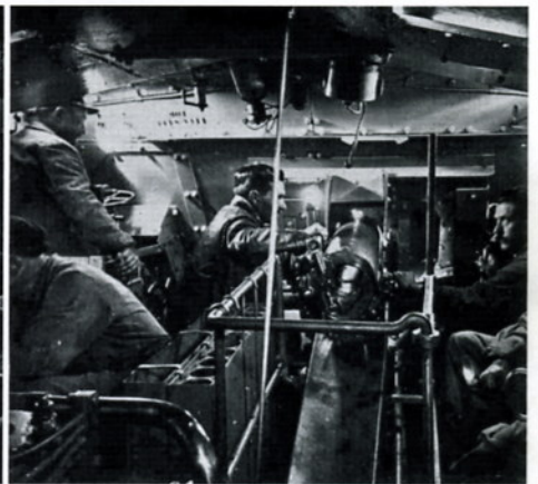
La Stéréoscopie Universelle (LSU) No. 0951, "Intérieur D'un Tank - Modele St Chamond" showing the interior of the St. Chamond heavy tank. It was armed with a very powerful 75 mm field gun and four machine guns. It was also slow, prone to breakdowns, and did not travel well over open terrain.
