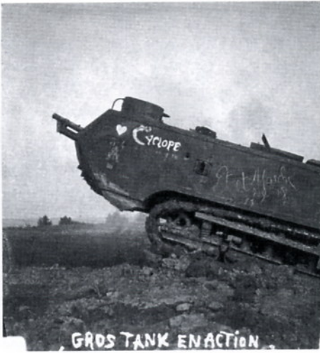
Enlargement from a 45 x 107mm glass stereo by an unknown French photographer showing a St. Chamond heavy tank named Cyclop. The 75mm gun prominent at the front of the tank was the most powerful gun ever mounted on a tank until WWII. The round commander's cupola is also prominent at the left front side of the tank. Note how far the front of the tank overhangs the treads. The rear also over hung the treads. This prevented the tank from crossing trenches or terrain full of shell holes. While the caption on the photo indicates that the tank is engaging the enemy, I doubt the photographer would have survived out in the open in No-Man's-Land to take a picture. This was most likely taken during a training exercise.
