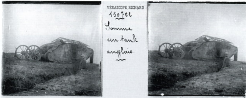
Verascope Richard No. 150762, "Somme un tank anglais" showing the 45 x 107mm glass view at actual size. Taken just after the battle of Flers in September 1916, where tanks were used for the first time, this is a Mark I with a broken track. It is a female version, armed only with machine guns. The male version carried 6-pounder guns, one on each side. The relaxed nature of the French soldiers, and their lack of gas masks, indicate the photo was taken well behind the front line. Note the pair of steering wheels at the rear. These were of dubious value and were left off of later models.
