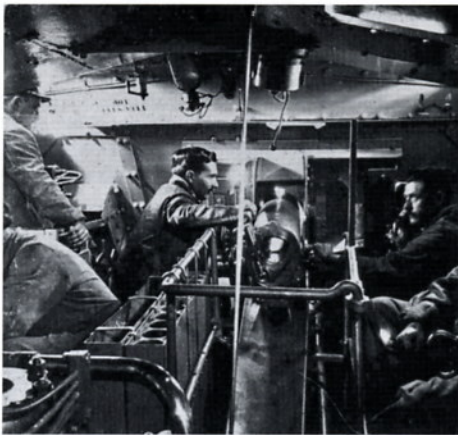
La Stéréoscopie Universelle (LSU) No. 0951, "Intérieur D'un Tank - Modele St Chamond" showing the interior of the St. Chamond heavy tank. It was armed with a very powerful 75 mm field gun and four machine guns. It was also slow, prone to breakdowns, and did not travel well over open terrain.
