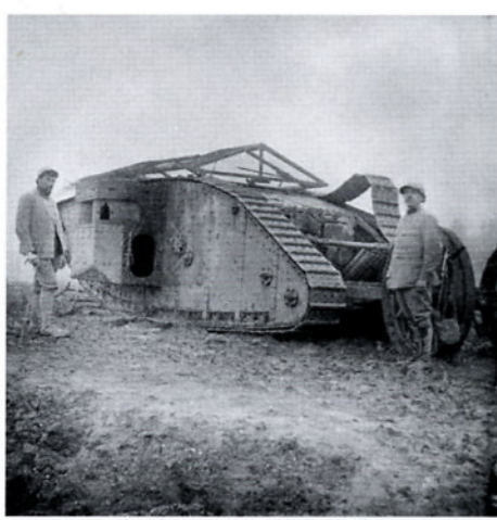
Verascope Richard No. 150764, "Somme un tank anglais" shows the same tank as No. 150762, the 45 x 107mm glass view reproduced here in a larger format. The structure on top of the tank is a wood frame covered in Chicken wire as a hand grenade defense. In theory, hand grenades thrown on top of the tank would roll off and explode harmlessly on the ground.
