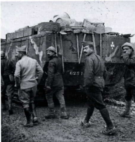
Enlargement from a 45 x 107mm glass view, "Gros Tank Francais." What may look like a garbage truck is actually the rear of a St. Chamond tank in use as a transport vehicle, clearly showing the long overhang.
