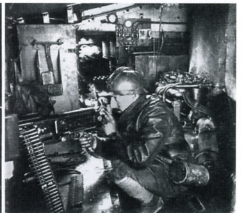
La Stéréoscopie Universelle (LSU) No. 01399, "Mitrailleur - Tank St. Chamond." Near this machine gun port, the engine can be seen open to the crew in the very cramped conditions. The use of flash for the photo greatly exaggerates the interior lighting level of the tank, which was normally very dark.
