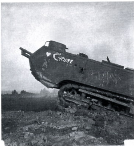
Enlargement from a 45 x 107mm glass stereo by an unknown French photographer showing a St. Chamond heavy tank named Cyclop. The 75mm gun prominent at the front of the tank was the most powerful gun ever mounted on a tank until WWII. The round commander's cupola is also prominent at the left front side of the tank. Note how far the front of the tank overhangs the treads. The rear also over hung the treads. This prevented the tank from crossing trenches or terrain full of shell holes. While the caption on the photo indicates that the tank is engaging the enemy, I doubt the photographer would have survived out in the open in No-Man's-Land to take a picture. This was most likely taken during a training exercise.
